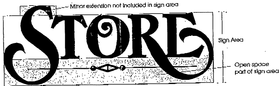
Figure 2. Calculation of open space area and area of minor extension
